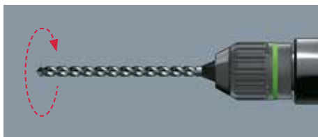
Rotary drilling: without percussion
